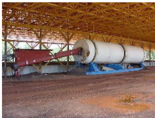
Figure A-14-2. In-Vessel composting is performed in an insulated silo, channel, or bin using a high-rate, controlled aeration system designed to provide optimal conditions. Rotating Drum Composters are a subset of in-vessel composters that aerate compost by turning the compost inside a rotating drum. Photo: Jason Governo, U. of Georgia
