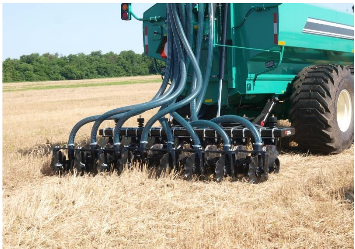
Figure A-17-2. Manure injection mechanically applies the organic nutrients – manure, bio-solids, or compost – into the root zone with surface soil closure at the time of application. This offers the greatest nutrient reduction and odor reduction due to limited soil disruption, amount of material left on the soil and immediate soil closure. Photo: Livestock and Poultry Environmental Learning Center (LPELC)
