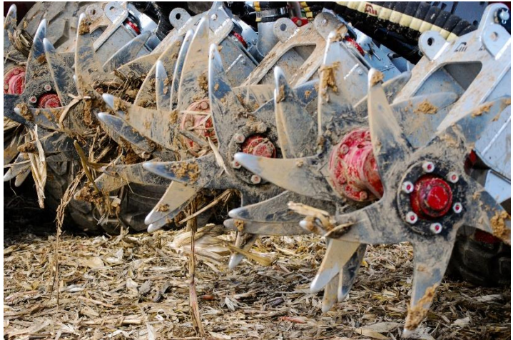
Figure A-17-1. Specialized equipment is used for manure incorporation and injection. Manure incorporation requires machinery that mixes dry, semi-dry or liquid organic nutrient sources – such as manure, bio-solids, and compost – into the soil profile. Photo: Chesapeake Bay Program
