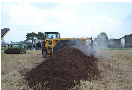
Figure A-14-4. Turned Piles and Windrows rely on frequent turning, usually with specialized machinery, to aerate the compost. Photo: Robb Meinen, Penn State
