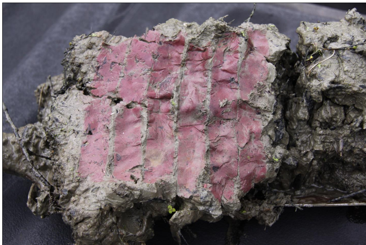
Figure 3. Example of a positive reaction to \alpha,\alpha' -dipyridyl dye, indicated by the development of a red or pink color following application of the dye onto a saturated soil containing \text{Fe}^{2+} in soil solution. This example used \alpha,\alpha' -dipyridyl dye test strips.
