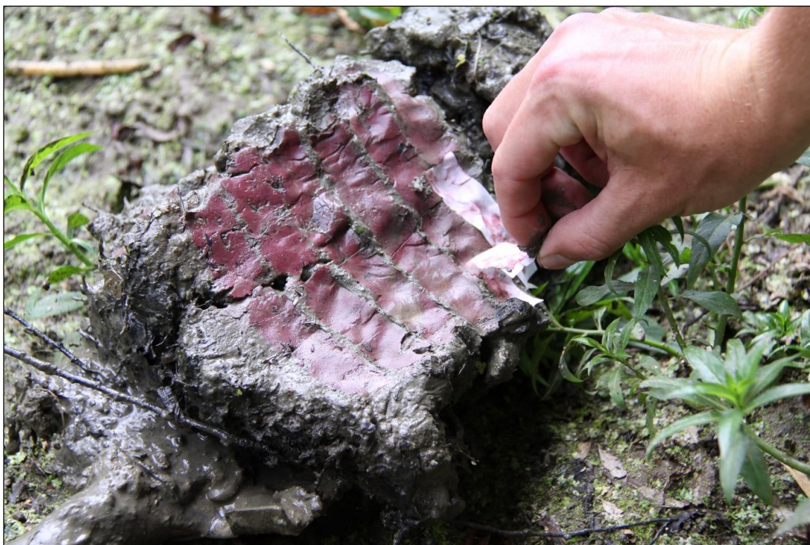
Figure 8. Example of \alpha,\alpha' -dipyridyl dye paper test strip application to a soil containing reduced iron ( \text{Fe}^{2+} ) in soil solution. Note that the reaction is clearly visible both on the soil surface and on the paper test strip and that the reaction occurs across more than 60% of the soil layer (Berkowitz et al. 2021).
