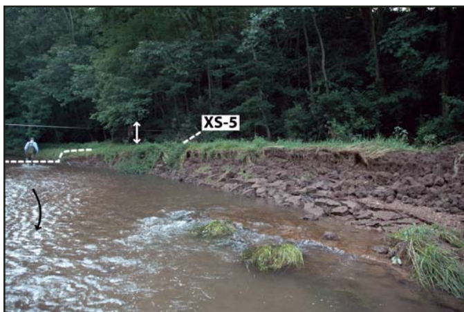
Figure 2. Mass movement occurred along the left bank of the incised Hammer Creek just downstream of XS 5 as a result of wetting and drying of the banks by high flow from a late June 2006 storm. Double arrow indicates person for scale along tape measure at section. Flat surface at top of bank is the level of sedimentation in the millpond. See Figure 5 for location of cross section.
